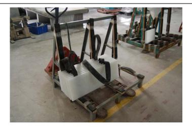
Separate each piece of **glass**<sup>2</sup> with a soft material (such as a rubber pad). This prevents vibration and human error, which helps eliminate inducing stress into the material.
