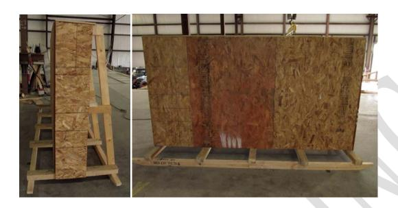
Finished crate should be free-standing, stabilized with internal and external bracing, and a rail system (runners) for ease of movement if crate is not continuously strapped down or in a rack system.
