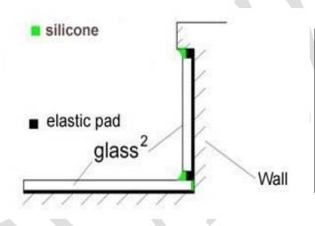
Vertical **glass**<sup>2</sup> must not contact with the horizontal **glass**<sup>2</sup> – both should be fixed directly to their wall surface. **glass**<sup>2</sup> is too heavy for direct contact as this will not allow for expansion hot weather. There should be a thick elastic pad (such as black rubber) between the two pieces and fill the gap with silicone.
